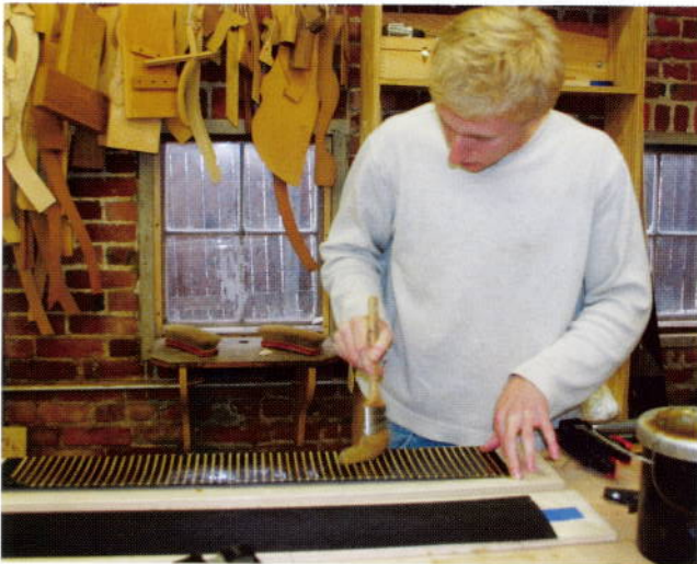
Fig. 17 Applying hot glue to the surface to re-melt excess glue residue
