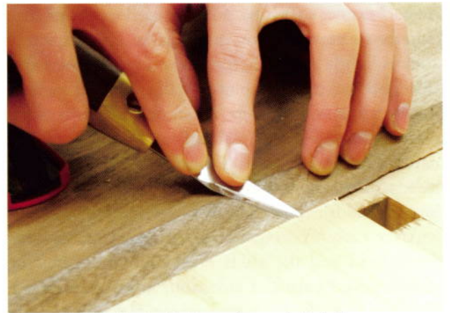
Fig. 12 Keep the knife flat to the angled block
