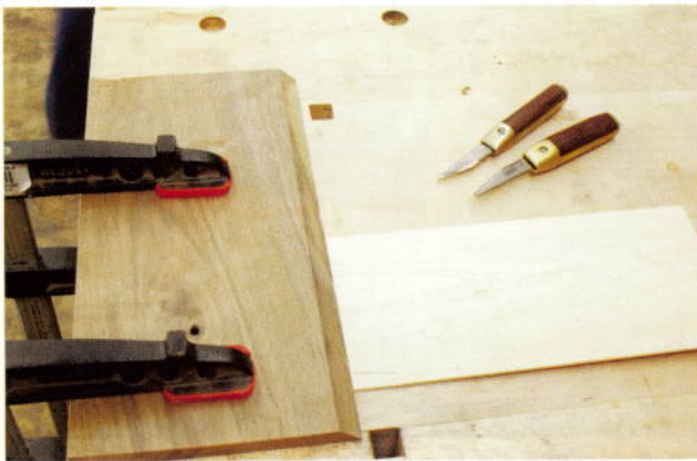
Fig. 11 Angle block (walnut) is clamped to the workpiece, indexed to the scribe line
